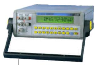
SN 8310 is a standard dc voltage and current source. It will supply voltages from 100 nV to 110 V and currents from 1 nA to 110 mA with an accuracy of better than 0,002% (20 ppm).
